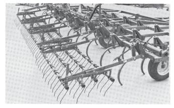
1a. The above 29' JD1610 chisel plow is shown with a 4 bar mounted harrow using M74 carrier arms. Two 7' sections were used in the center and one 8' section was used on each wing. An optional method is to use one 14' section in the center with 3 carrier arms. Wing section sizes will vary with the width of the chisel plow.
